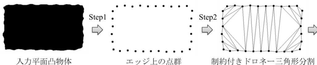
Fig.1 Constrained Delaunay Triangulation (Step1,2,3)
